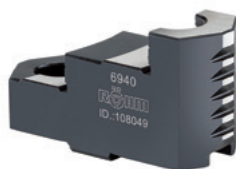
A09 Reversible top jaws UB, DIN 6350, hardened tongue and groove for external and internal clamping, material 16 MnCr5
