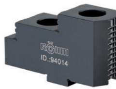
A28 Reversible top jaw UB, 3-jaw set, hardened tongue and groove for external and internal clamping, material 16 MnCr5
