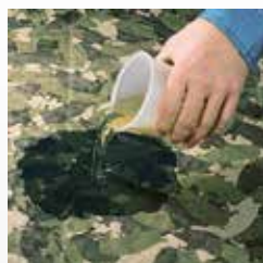
225 ml oil is poured onto the HAM-O...
