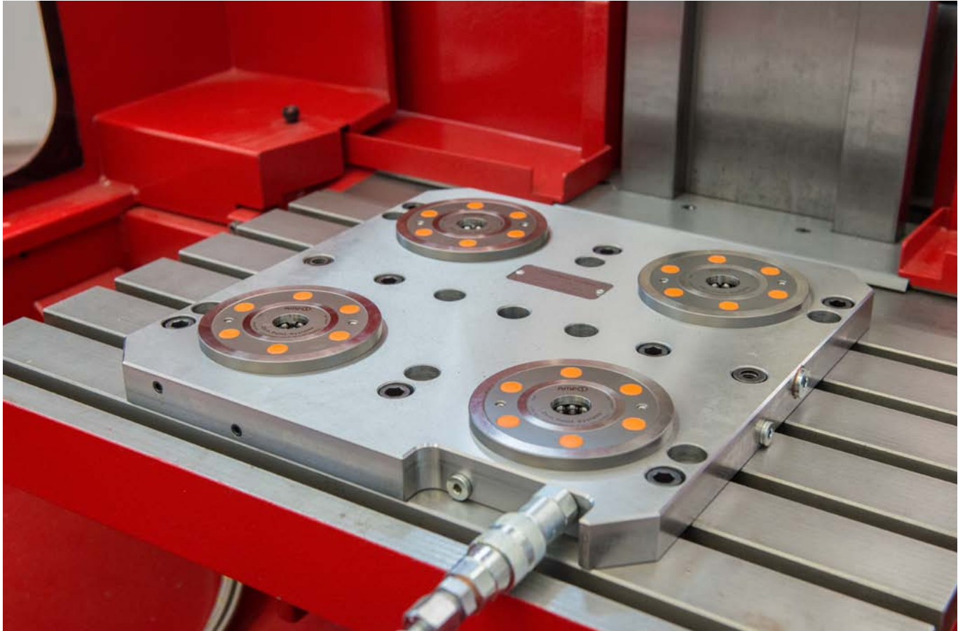
Use of various sizes of standard clamping modules in one application.
