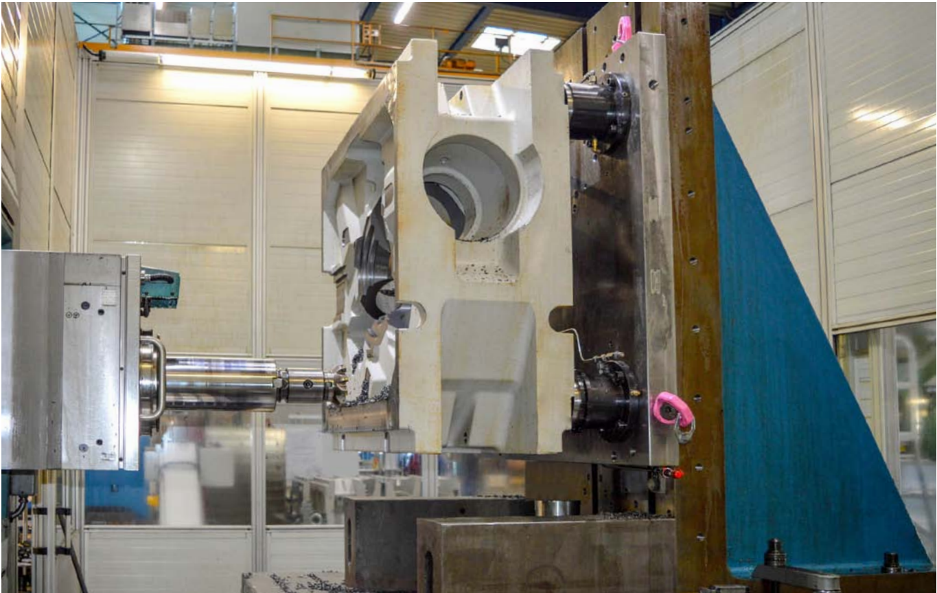
Direct clamping of the workpiece on a horizontal machining centre.
