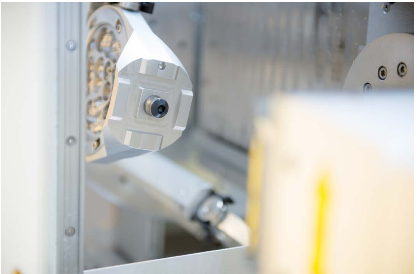
Our zero-point system is the factory standard interface here between the machine table and blank carrier.
