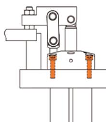
From above with 4 socket cap screws through the flange.
