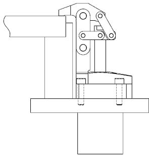
From above with 4 socket cap screws through the flange.
