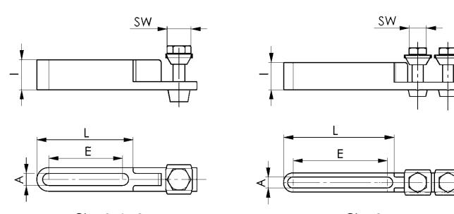
**No. 6878K****Clamping bolt for perforated tables**
