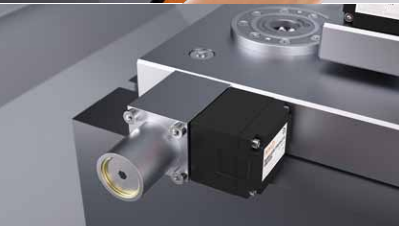
3 Hydraulic pressure monitoring by means of the integrated radio pressure switch. This monitors in this case the system pressure of the hydraulic zero point clamping station.
