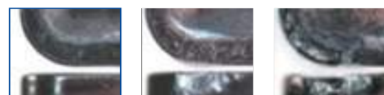
AC420K (Left): Shows minimal edge wear. Competitor's Product D (K15) (Middle): Shows significant edge wear. Competitor's Product E (K20) (Right): Shows significant edge wear.
