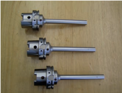
HSK-A100 x \varnothing 10 x \varnothing 23 x 260 Art.-Nr. 4004-422.00
