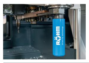
After the lubrication process, Lubritool® is sent back to the tool magazine and remains there until the next lubrication cycle.
