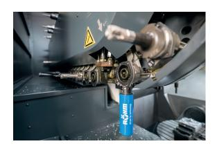
Lubritool® is located in the tool magazine. Whenever the machine control notifies that a lubrication process is necessary, Lubritool® will be sent up into the spindle.
